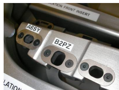
Stickers identifying the checking fixture RPS (foreground) as well as a removable block (background)
