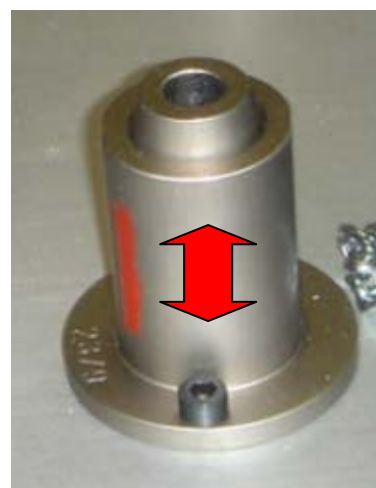
Conic centring pin, enabling to center the part on one of its holes; the shape of the centring pin allows to absorb the hole manufacturing tolerance to center the part in a optimum way.
